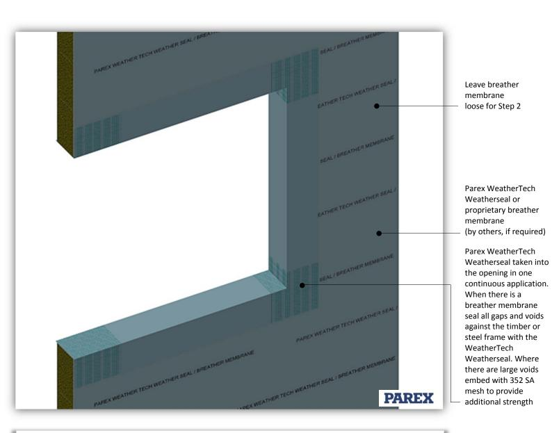
The general principles of this detail will apply to all forms of openings. For unusual applications contact Parex for additional guidance.
