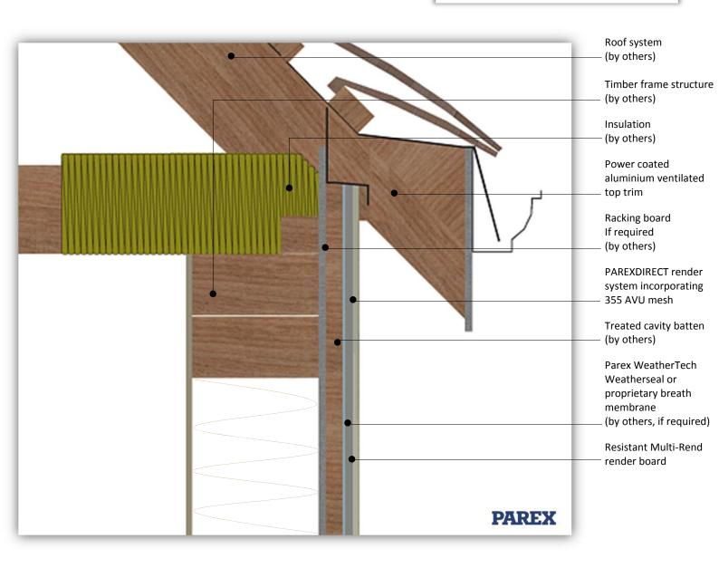
System: PAREXDIRECT onto Timber Frame
