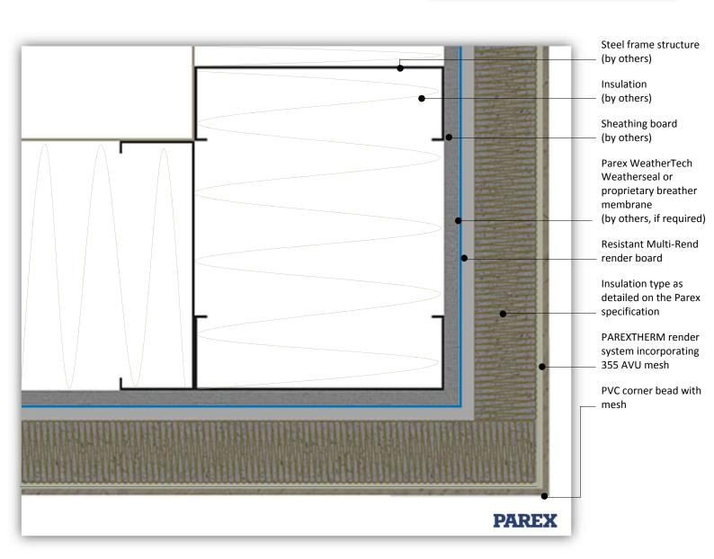
System: PAREXTHERM onto Steel Frame
