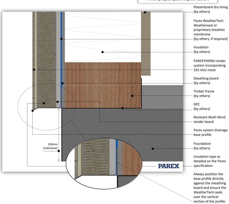
System: PAREXTHERM onto Timber Frame
